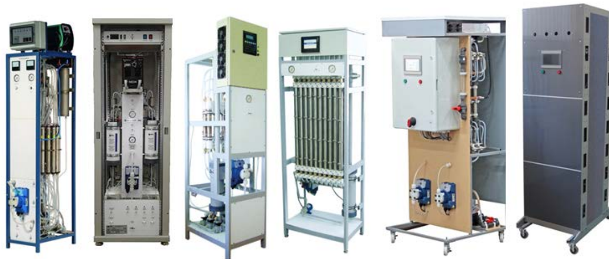
Fig. 10. AQUACHLOR and ECOCHLOR devices, from left to right: AQUACHLOR-500 (A-500) with a capacity of 500 grams of chlorine gas per hour, requires frequent cleaning of the electrochemical reactor with hydrochloric acid, 2005; installation of A-500M, 500 grams of chlorine gas per hour, equipped with self-cleaning reactor, manual control of working parameters, 2012; A-600 and ECOCHLOR-3000 (E-3000) devices with a capacity of 600 and 3000 grams of chlorine gas per hour, reactors with the MB elements of a new generation, semi-automatic control, 2016; A-800 and E-4000 devices with chlorine gas capacity of 800 and 4000 grams per hour, self-cleaning reactors, remote monitoring and control, 2017.
