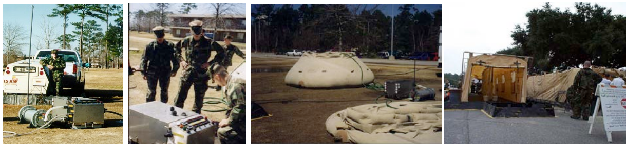
Fig. 2. Marines at the training range deploy the mobile device "Decontamination Generator" with FEM-3 (MB-11) elements, filling the rubber-fabric tanks with anolyte ANK and treatment with anolyte of military personnel, their equipment and weapons in the tent where the shower systems are installed. Atlanta, USA, 2001.
